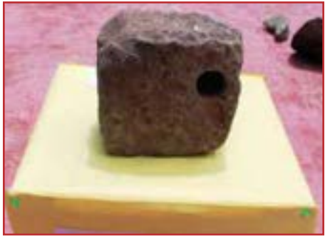
Dressed stone used for construction of fort Lohgarh. There is hole in every stone so that lime mortar can get its strength and each stone are bound with other one strongly.
